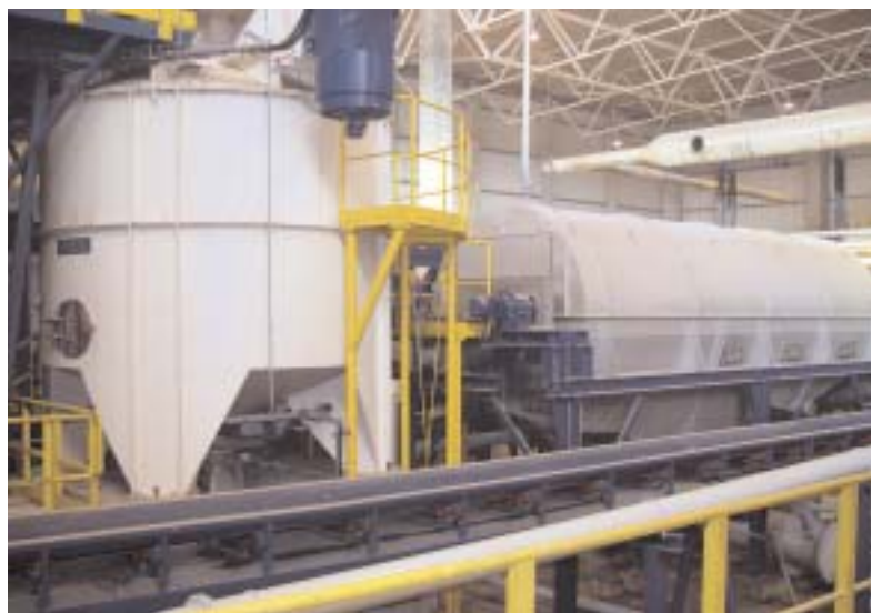
Pulper unit for removal of settleable and floating impurities from biowaste in wet fermentation processes (Picture courtesy of LINDE KCA, Germany)
