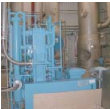
Water wash is one of the most common techniques for separating carbon dioxide from biogas.
